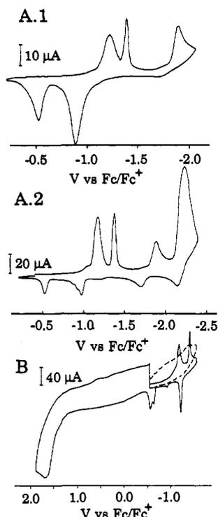
**Figure 2.** Cyclic voltammograms of a film of  $C_{60}$  on a platinum electrode (1-mm diameter) in a solution of MeCN [supporting electrolyte: 0.1 M (TBA)BF<sub>4</sub>] showing (A) (1) third reduction; (2) fourth reduction; and (B) oxidation processes. Solid curve, first scan; dashed curve, second scan;  $v = 200$  mV/s.
