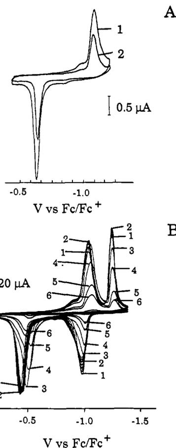
Figure 1. Cyclic voltammograms of a film of  $\text{C}_{60}$  on a platinum electrode in a solution of MeCN; supporting electrolyte: 0.1 M (TBA)AsF<sub>6</sub>. Reversible reduction processes: (A) First reduction. (1)  $v = 200$  mV/s; (2)  $v = 100$  mV/s. (Electrode diameter: 250  $\mu\text{m}$ ). (B) Second reduction and effect of continuous scanning at 200 mV/s. (1) First cycle; (2) 10th cycle; (3) after 5 min; (4) after 10 min; (5) after 20 min; (6) after 25 min. (Electrode diameter: 1 mm.)
